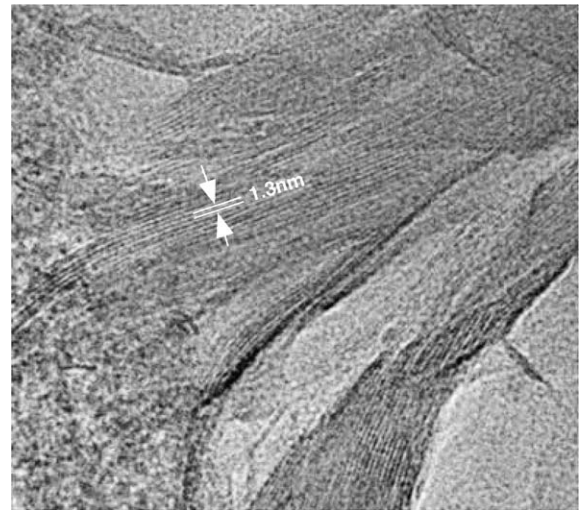
Fig. 7. Higher magnification view of the fibrous phase (Area 1 in Fig. 6) in the altered glass from Test 1 with 0.1 M NaOH solution at 150 °C for 30 days.
